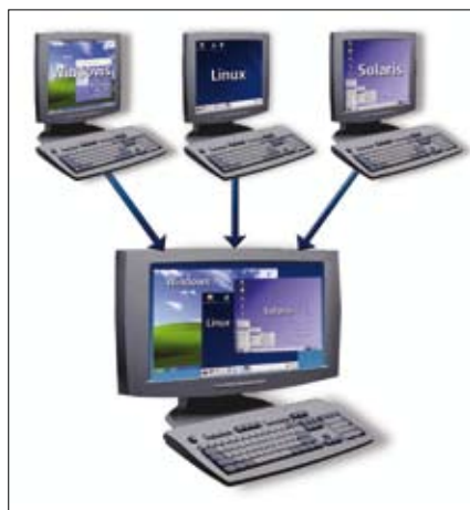
Fig 1: Virtual IT enables multiple operating environments to run on a single hardware platform.
