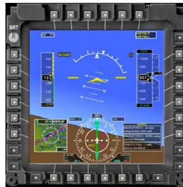
**Real-Time Avionics Display Rendered on Freescale Platform remotely controlled on a WindowsXP System**
